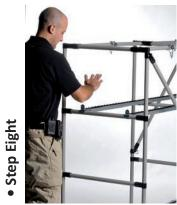
Insert long rollers on remaining tiers. Lightly tap rollers into position.
