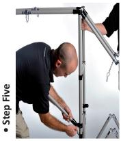
Insert locking pin into side support arm. Repeat steps 2-5 for the other half of rack. Make sure that all pins are secured.
